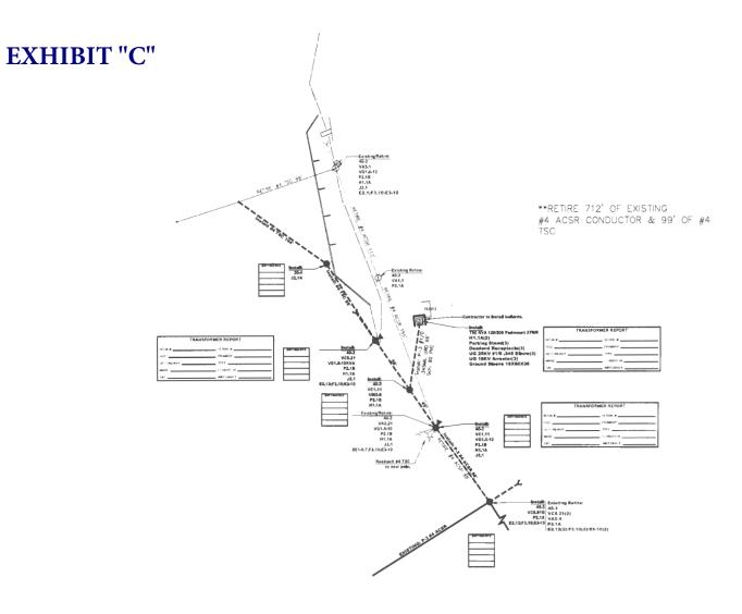
\*Concrete Pcd, GRC Sweep Elbows, Ground Sleeve, high lugs, riser, bolloras & Grounding Bushings to be installed by contractor
